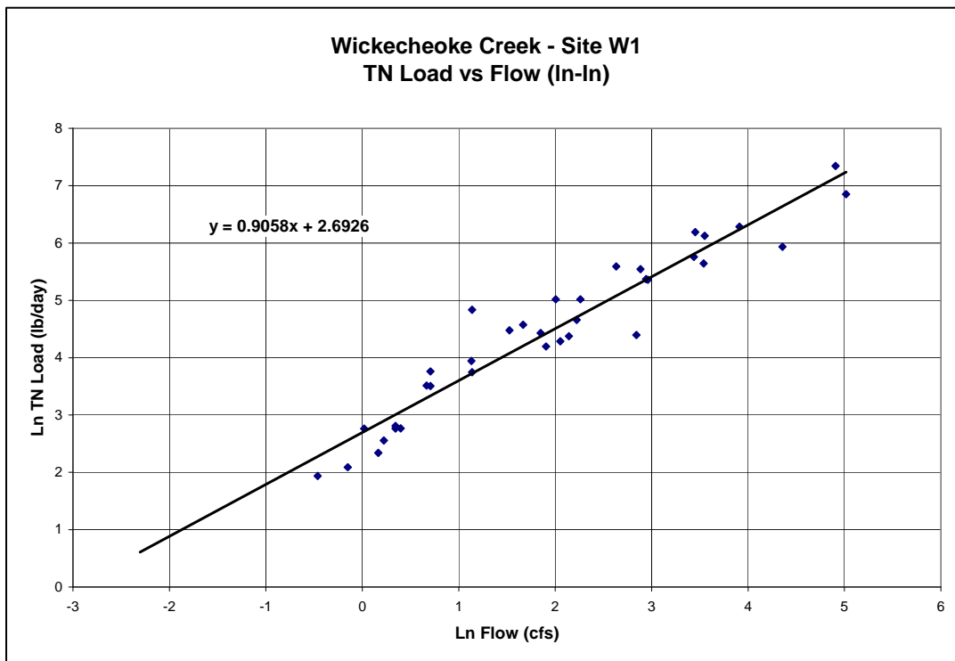
Figure 7: Relationship (natural ln-ln) of total nitrogen (TN) load to flow for site W1 on Wickecheoke Creek
