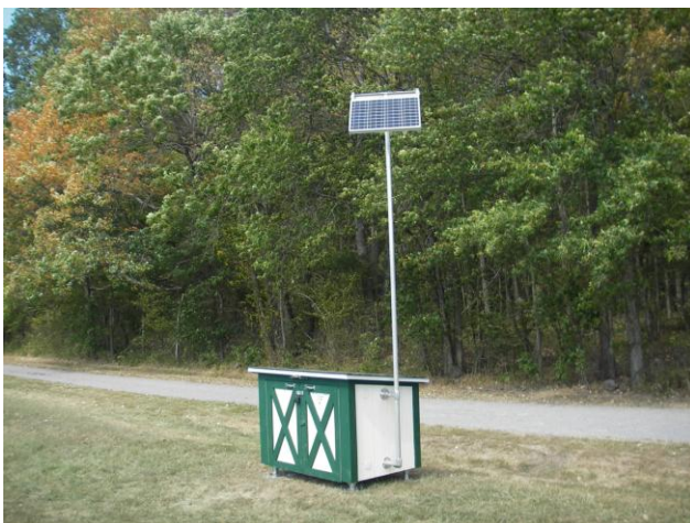
Sampler housing with solar panel.
